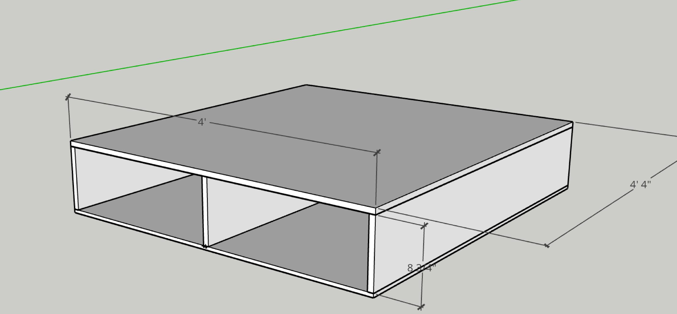
The vertical supports and top of the frame is made out of 3/4" Plywood. The bottom of the frame is 1/2" plywood in order to save on weight. In the final build I used slats on the
